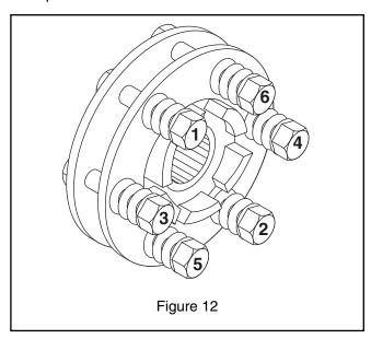
**NOTE:** Do not tighten the bolts in a circular sequence, that is, by tightening the bolt next to one which was just tightened. The bolts should be tightened in a cross sequence, that is, by tightening one bolt, then tightening the bolt which is across from it on the plate. Continue tightening the bolts in this sequence until all the bolts are tightened. (Figure 12)
